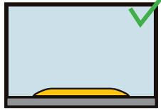
Superior Mark's **beveled edges** allow for objects to easily roll or pull over the floor marking with less damage, or releasing from the floor.
