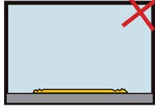
**Sharp edges** make it more difficult for objects to roll or pull over the floor marking. They are more prone to damage or releasing from the floor.
